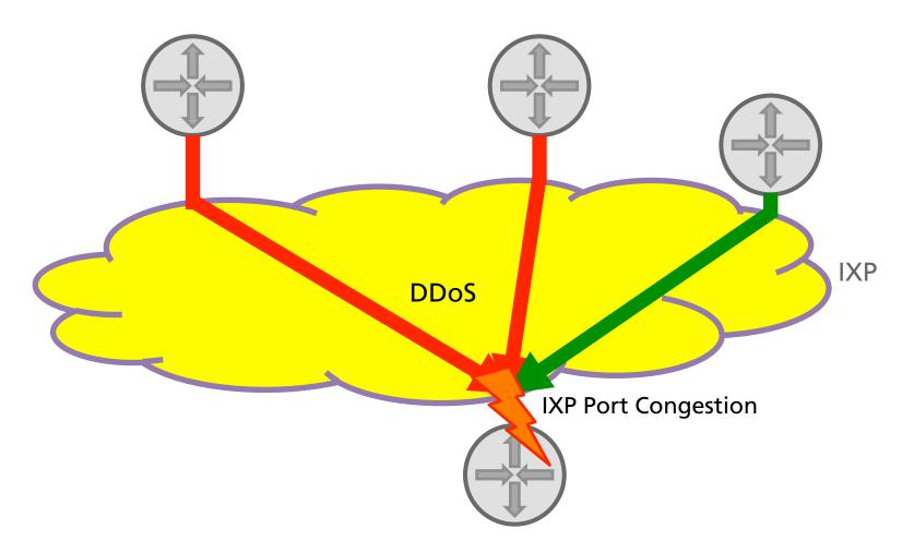
If an IXP customer is hit by a massive DDoS attack its port can get congested and impact legitimate traffic
